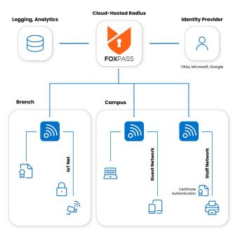
The above is a high-level representation of a typical SMB or Education deployment. Set up and management of the systems is simple and supports both username/password and passwordless authentication. The solution supports multiple SSIDs, devices, staff, and guest access. Detailed logs are available for comprehensive monitoring and compliance requirements.
